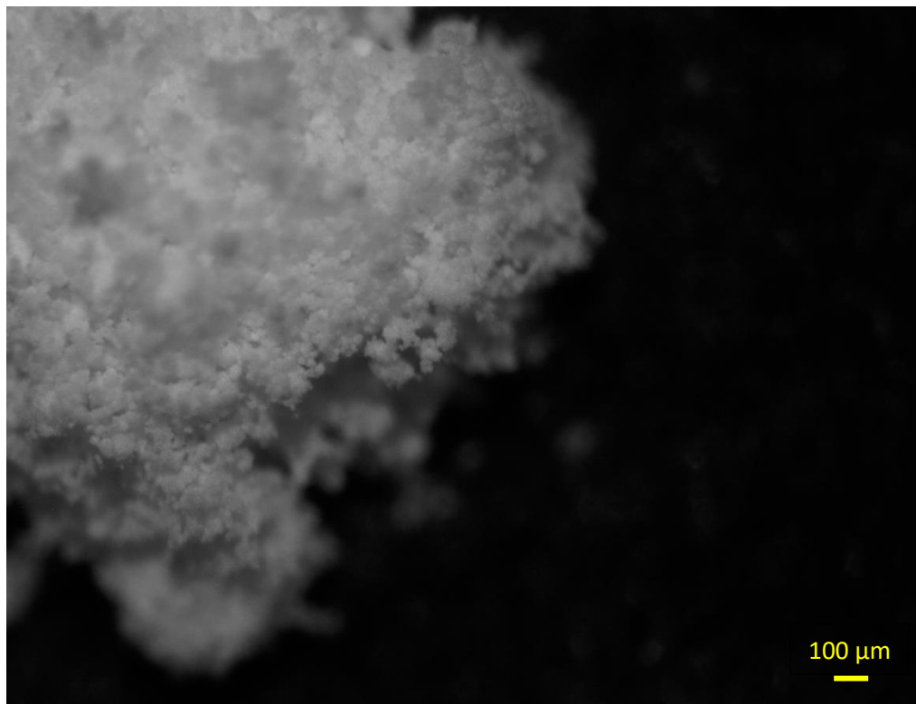
Figure S.1: MgO powder observed by optical microscopy on a cardboard surface.
